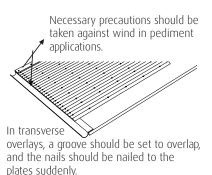
If the slope is 21% and above; Newoline Plate; 970/2000 mm Newoline Roof Ridge; 48.5x2000 mm Wood Purline; 5/8 Galvanized Plastic-Headed Mono-bloc Nail; 8 cm Wooden Rafter
